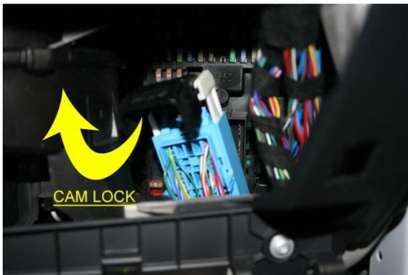
Disconnect the 2 Grey Connectors from the bottom of the CJB. Remove the 2 10mm nuts. While pulling the CJB partially out, reach up behind and unplug both connectors held by CAM Locks. They are also Green and Orange, but smaller:
