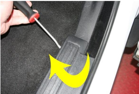
Pull back the felt weather-strip from the A-Pillar:
