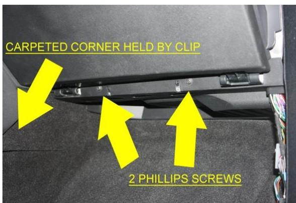
Push the 2 plastic hinge pins towards the center and then remove the glove compartment:
