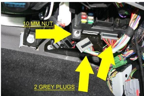
The large Blue Connector and 2 Grey Connectors can be pulled through the glove compartment opening for easier access. Maneuver the CJB out of the dash:
